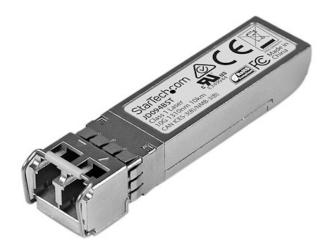
The JD094BST is an HPE JD094B compatible fiber transceiver module that has been designed, programmed and tested to work with HPE brand switches and routers. It delivers dependable 10 GbE connectivity over fiber cable, for 10GBASE-LR compliant networks, with a maximum distance of up to 10 km (6.2 mi).
