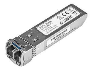
The SFP10GLRST is a TAA compliant Cisco SFP-10G-LR compatible fiber transceiver module that has been designed, programmed and tested to work with Cisco brand switches and routers. It delivers dependable 10 GbE connectivity over fiber cable, for 10GBASE-LR compliant networks, with a maximum distance of up to 10 km (6.2 mi).
