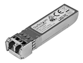
The SFP10GSRXST is a Cisco SFP-10G-SR-X compatible fiber transceiver module that has been designed, programmed and tested to work with Cisco brand switches and routers. It delivers dependable 10GbE connectivity over fiber cable, for 10GBASE-SR compliant networks, with a maximum distance of up to 300 m (984 ft.).
