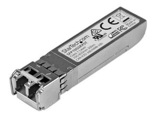
The SFP10GSRXST is a Cisco SFP-10G-SR-X compatible fiber transceiver module that has been designed, programmed and tested to work with Cisco brand switches and routers. It delivers dependable 10GbE connectivity over fiber cable, for 10GBASE-SR compliant networks, with a maximum distance of up to 300 m (984 ft.).
