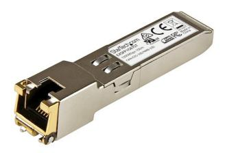
The EXSFP1GETST is a Juniper EX-SFP-1GE-T compatible copper transceiver module that has been designed, programmed and tested to work with Juniper brand switches and routers. It delivers dependable 1 GbE connectivity over copper cable, for 10BASEBASE-T, 100BASE-TX and 1000BASE-T compliant networks, with a maximum distance of up to 100 m (328 ft.).
