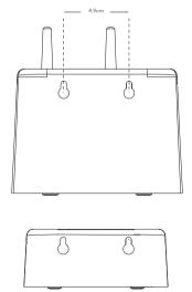
Insert the wall plugs if necessary, then insert the screws leaving about 5mm protruding from the wall on which to hang the phone.
