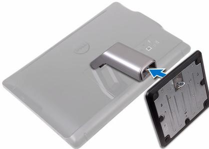
c) Tighten the captive screw to secure the base to the stand riser.
