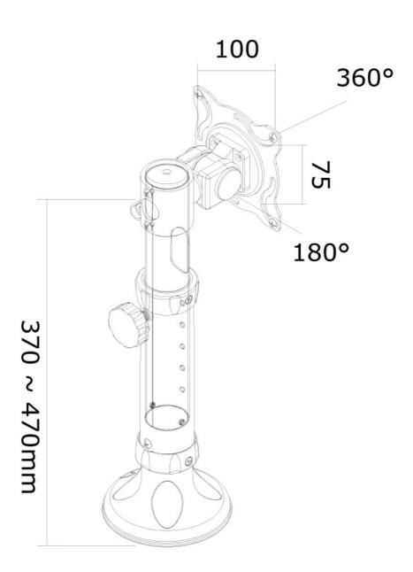
Neomounts Measuring unit: mm
