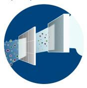
With cutting edge sensing and purification technology, the Philips Air Purifier Series 2000 is proven to reduce allergens, odors, VOCs and even certain bacteria. The pre-filter and True HEPA filter remove particles. The Active Carbon filter reduces gases and odors.
