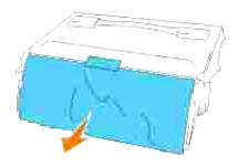
2. To insert the drum cartridge, push up the lever on the right side of the printer. With the lever in the upright position, hold the drum cartridge by the handle, align the arrows on the drum cartridge with the corresponding arrows on the printer and guide the cartridge in until it snaps into place.
