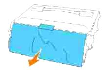
2. To insert the drum cartridge, push up the lever on the right side of the printer. With the lever in the upright position, hold the drum cartridge by the handle, align the arrows on the drum cartridge with the corresponding arrows on the printer and guide the cartridge in until it snaps into place.
