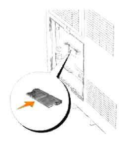
5. Reattach the control board cover to the printer.
