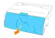
3. To insert the drum cartridge, push up the lever on the right side of the printer. With the lever in the upright position, hold the drum cartridge by the handle, align the arrows on the drum cartridge with the corresponding arrows on the printer and guide the cartridge in until it snaps into place.
