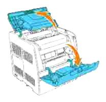
2. To remove the used drum cartridge, push up the lever on the right side of the printer.
