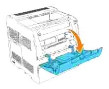
2. Push up the handhold on the right to unlock the cartridge.
