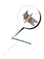
4. Hold the new cleaning pad under the cleaning rod and push it in until it clicks.
