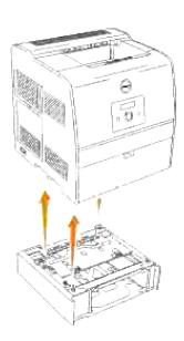
6. Attach the trays together by installing the optional tray you just removed on top and inserting the two screws provided. Tighten the screws until they are secure.
