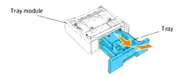
2. Place the tray module in the location that you would like the printer to be located.
