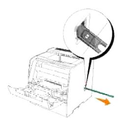
3. Push the two tabs on the cleaning pad inward to remove the pad.
