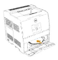
To load envelopes that are under 8.66 inches (220 mm) in width, insert the envelopes with the flaps open and toward the front of the printer, with the recommended print side face up.
