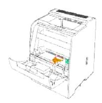
2. Pull the cleaning rod until the cleaning pad comes out of the printer.
