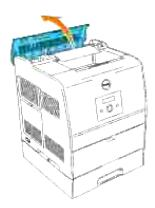
3. Press the levers on both sides and remove any jammed print media.
