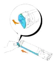
3. To insert the toner cartridge, face the label on the cartridge to the front and align it with the arrows on the printer.
