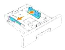
3. Squeeze the length guide and slide it to the front edge of the tray.
