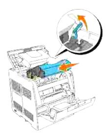
4. Pull down the lever on the right to lock the drum cartridge in place.
