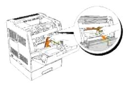
3. Make sure the color of the toner cartridge matches the slot on the toner cartridge carrier. The order is Y, M, C, K. Gently shake the cartridge to distribute the toner evenly.
