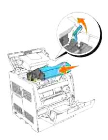
3. Pull down the lever on the right to lock the drum cartridge in place.
