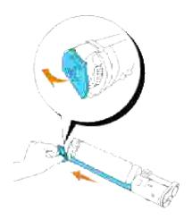
6. To insert the toner cartridge, face the label on the cartridge to the front and align it with the arrows on the printer.
