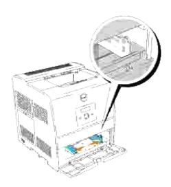
3. Insert the print media into the feeder with the recommended print side face up.
