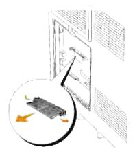
4. Reattach the control board cover to the printer.
