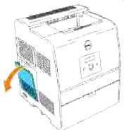
3. Hold the memory card so the notch is aligned with the projection on the slot.
