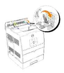
CAUTION: Never touch the outer levers located on both sides of the fuser unit, which are used to remove or install the fuser unit.
