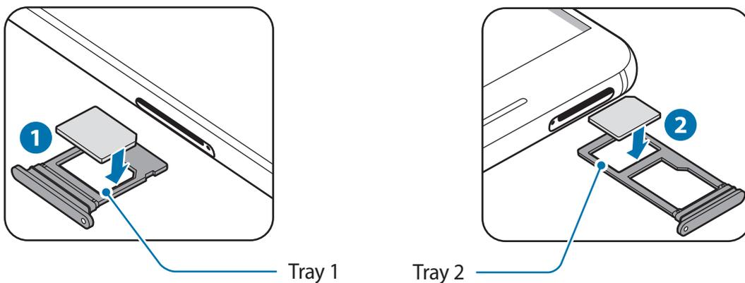
**4** Gently press the SIM or USIM card into the tray to secure it.
