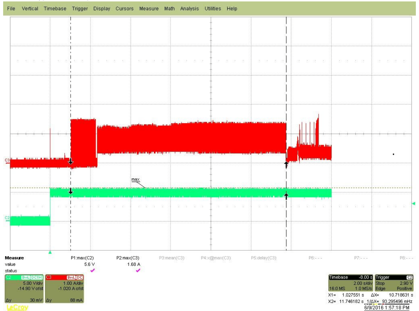
Figure 1. 10TB & 8TB - Typical 5V and 12V startup and operation current profiles
