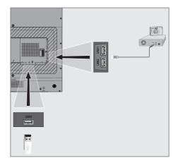
Connect the USB1 or USB2 USB interface on the television and the related data output on the external device (external hard disk, digital camera, card reader or MP3 player) with a USB cable;
