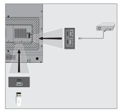
Plug the external hard disk to the USB1 or USB2 USB interface of the television;
