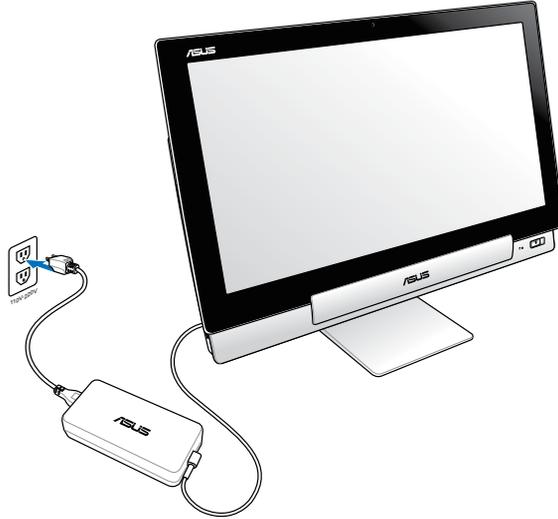
1. Connect the power adapter to your PC Station's DC-in port and plug to the correct socket outlet with the correct input rating. The input voltage of the adapter is 100Vac~240Vac.
