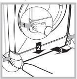
**2.** Loosen the drainage pump cover by turning it anticlockwise: it is normal for some water to leak out;
