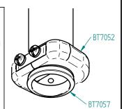
To use the larger BT7051 collar, new safety bolt holes must be drilled at least 27mm from the end of the pole to allow the Pole End Ring to fit on.
