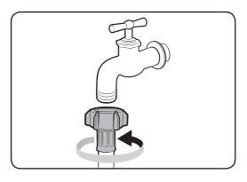
• If using a screw type of water tap, connect the water hose to the water tap as shown.
