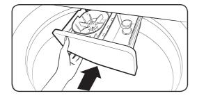
**5.** When complete, close the rinse cap and reinsert the distributor. Then, reinsert the detergent drawer.
