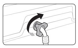
**7.** Connect the other end of the water hose to the inlet valve on the back of the washing machine. Turn the hose clockwise to tighten.
