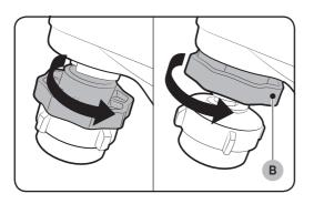
**3.** When levelling is complete, tighten the nuts (B) if provided (some models may not have the nuts).
