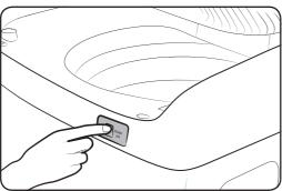
Water Jet and Built-in sink help you handwash before the washing machine starts operation. Water Jet is available only when the door is open with the water level set to less than High. For prewashing, use the Built-in sink that is designed to facilitate the hand-wash.
