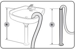
2. Connect the other end of the drain hose to a standpipe or basin that is positioned 90-100 cm (\*) from the floor.
