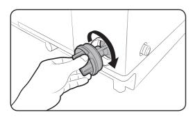
3. Reinsert the filter, and turn clockwise until it locks into position.
