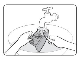
**4.** Clean the drawer as well as the distributor and rinse cap with running water and a soft brush.
