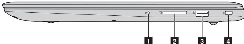
**1 Novo button** When the computer is off, press this button to start the System Recovery or the BIOS setup utility, or to enter the boot menu.
