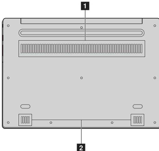
**1** **Ventilation slots** Dissipate internal heat.
