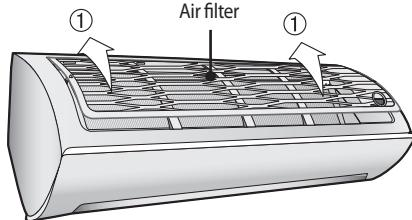
2. There's one hook at both sides of the filter, press the surface of the Air filter softly and get the hooks into the main body. ②
