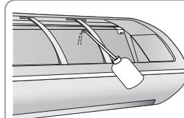
After completing the installation of the drain hose, pour water into the drain pan to check whether the hose is well drained.
