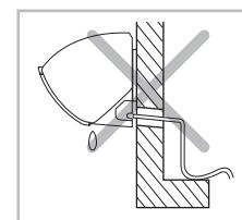
The drain hose must not be bent.
