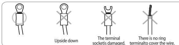
► There must be no space between the terminal and the screw when connected.
