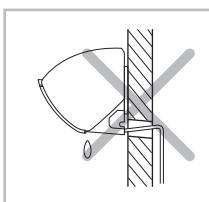
The drain hose must NOT slant upwards.
