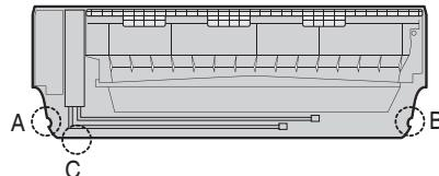
1. Cut out the appropriate knock-out piece (A, B, C) on the rear of the indoor unit unless you connect the pipe directly from the rear.
