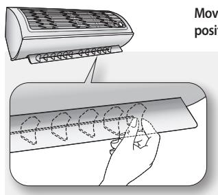
Move the blade pin lever left or right to keep the air flow direction in a constant position you prefer.
