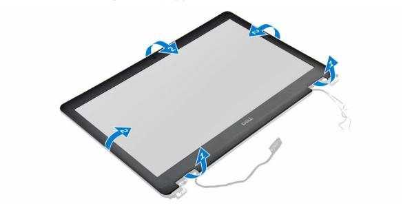
4 Remove the display bezel from the display assembly.
