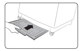
The washing machine comes with the Antirat panel that protects small animals such as rats from entering the machine. Insert the panel into the bottom of the machine. To facilitate the work, slightly lift up the bottom front.
