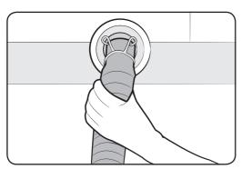
Insert the drain hose into the drain outlet. Make sure to connect them firmly using the joint ring. The drain hose is extensible. Adjust the length of the drain hose as needed.
