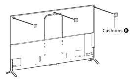
Make sure that the wall has enough space for the TV and is capable of supporting a weight of at least four times that of the TV.
