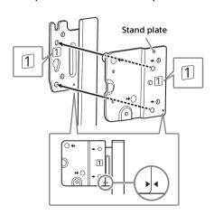
3 Fix the stand plate to the Table-Top Stand with screws (M5×10) (supplied with the TV).
