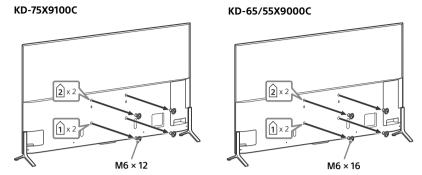
3 Attach the U-shaped Bar **⑤** (supplied with the TV) to the rear of the TV. KD-75X9100C
