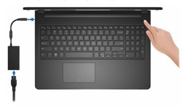
Figure 1. Connect the power adapter and pressing the power button
