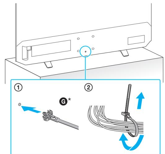
**Installation** Do not bundle the AC power cord (mains lead) together with other cables.
