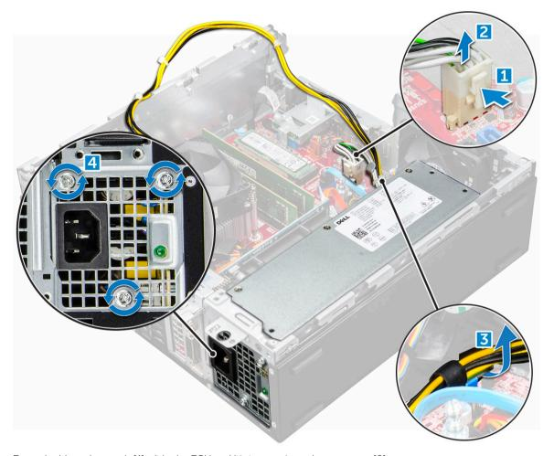
Press the blue release tab [1], slide the PSU and lift it away from the computer [2]. 5
