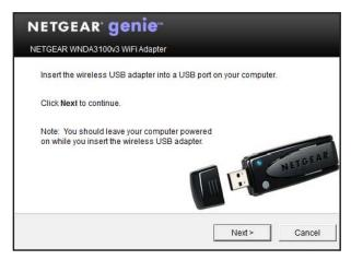
5. Insert the adapter into a USB port on your computer with or without the USB cable and plastic cradle.
