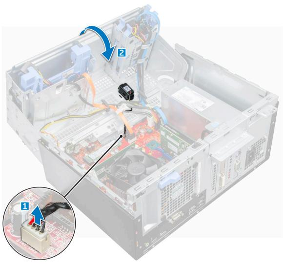
c  $\,\,$  Press the release tabs [1], and slide the speaker [2] out of the slot.
