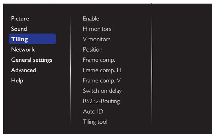
With this function you can create a single large-screen matrix (video wall) that consists of up to 100 sets of this display (**up to 10-sets on the vertical and 10-sets on the horizontal sides**).
