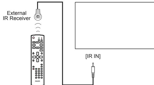
NOTE: This display's remote control sensor will stop working if the [IR IN] is connected.
