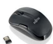
The Wireless Mouse WI200 uses the latest wireless 2.4 GHz technology, and a high-resolution 1000 dpi optical sensor to give you the precision and reliability you need. Sporting a compact design with a stylish black finish, the WI200 wireless mouse is well suited to all environments and to each user whether right or left handed.
