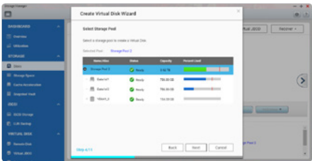
Step 3: Check the available space and create a virtual disk.
