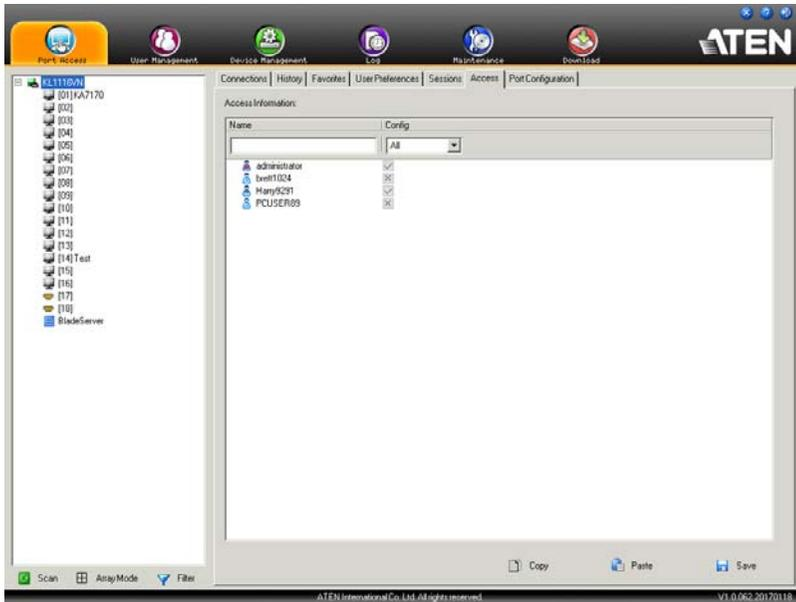
The page is essentially the same as the one for the Browser GUI (see page 119), with the exception that there are filters at the top of the columns. The filters allow you to expand or limit the scope of the users and groups that are displayed, as described in the following table:
