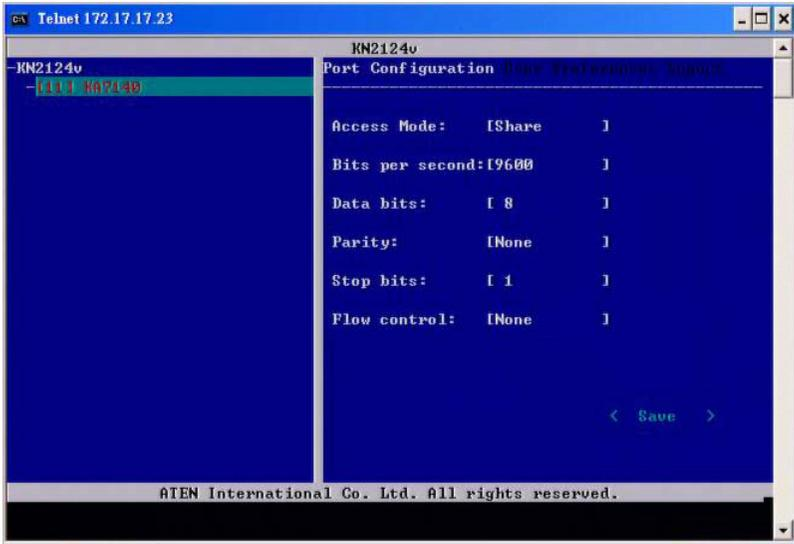
The configuration settings that can be made when a serial interface device is selected are described in the table, below:
