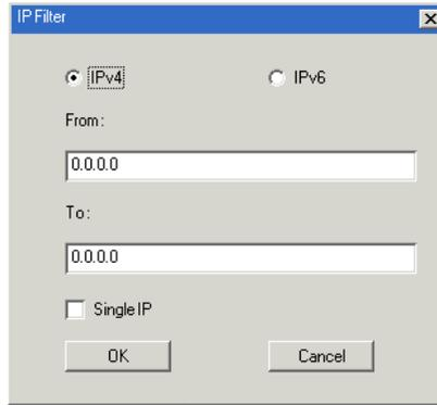
2. Specify whether you are filtering an IPv4 or IPv6 address.
