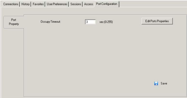
The Occupy Timeout field sets a time threshold for users on ports whose Access Mode has been set to Occupy (see *Access Mode*, page 127). If there is no activity from the user occupying the port for the amount of time set here, the user is timed out and the port is released. The first user to send keyboard or mouse input after the port has been released gets to occupy the port.
