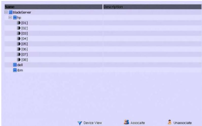
Blade View lists all of the blade servers (IBM and Dell servers) and individual blades (HP servers) that are installed on the system, and the ports (if any) that they are associated with.
