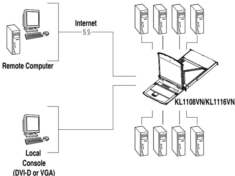
For added convenience, ports for an external keyboard, monitor (DVI-D or VGA), and mouse are provided on the rear panel – permitting you to manage the switch from a local console. There is also an external USB mouse port on the keyboard module, allowing you to use an external mouse, rather than the touchpad.
