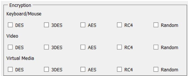
The screenshot shows a window titled "Encryption" with three sections: "Keyboard/Mouse", "Video", and "Virtual Media". Each section contains five checkboxes for encryption methods: DES, 3DES, AES, RC4, and Random.
