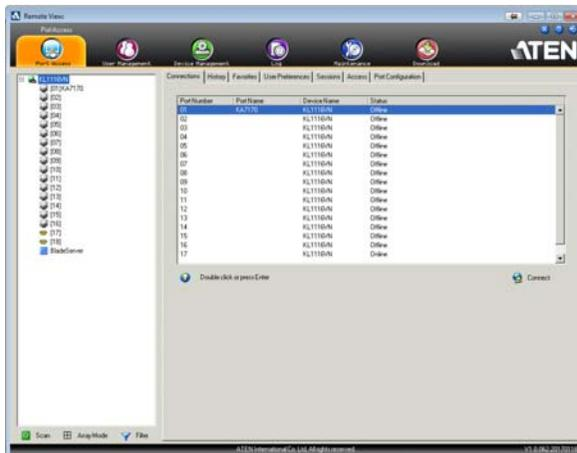
The Connections page is organized into several main areas. All the devices, ports, and outlets that a user is permitted to access are listed in the Sidebar at the left of the page. In addition to KVM over IP device listings, if any PON (Power Over the Net™) devices are connected to the switches they are listed separately below the switch listings. If any Blade Servers have been deployed, they are listed separately below the PON devices.
