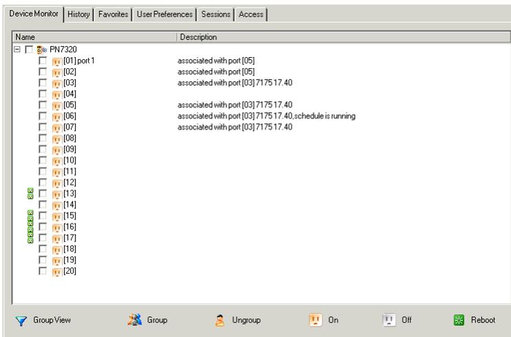
PON View is the default page view, All PON devices and their outlets that are connected to the switch are listed under the *Name* column.
