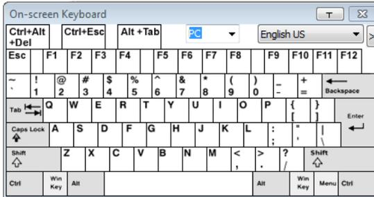
One of the major advantages of the on-screen keyboard is that if the keyboard languages of the remote and local systems aren't the same, you don't have to change the configuration settings for either system. Just bring up the on-screen keyboard; select the language used by the server you are accessing; and use the on-screen keyboard to communicate with it.
