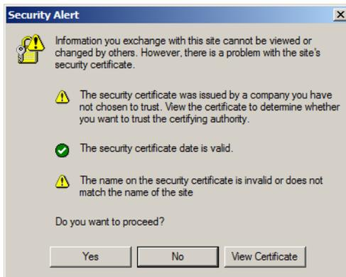
The certificate can be trusted, but the alert is triggered because the certificate's name is not found on Microsoft's list of Trusted Authorities. You have two options: 1) you can ignore the warning and click **Yes** to go on; or 2) you can install the certificate and have it be recognized as trusted.
