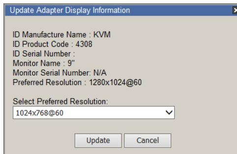
Use the *Display Information* button to obtain the local monitor's Preferred Resolution (optional), and apply it with the *Select Preferred Resolution* drop down menu, then click **Write**. If the local console is not connected to a monitor, the default EDID setting is loaded on the adapter cable.
