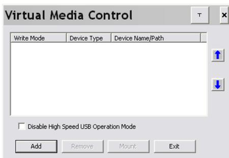
**Note:** The T button at the top right brings up a slider to adjust the transparency of the dialog box. After making your adjustment, click anywhere in the dialog box to dismiss the slider.
