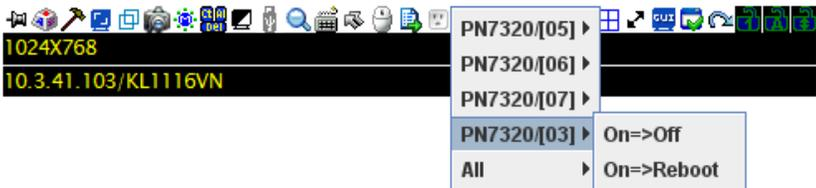
After clicking on the PON icon, a list of the power outlets associated with the connected port appears with the available options:
