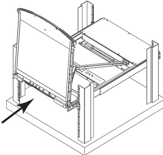
3. Rotate the LCD module all the way down, then pull the rear catches to release the LCD module.
