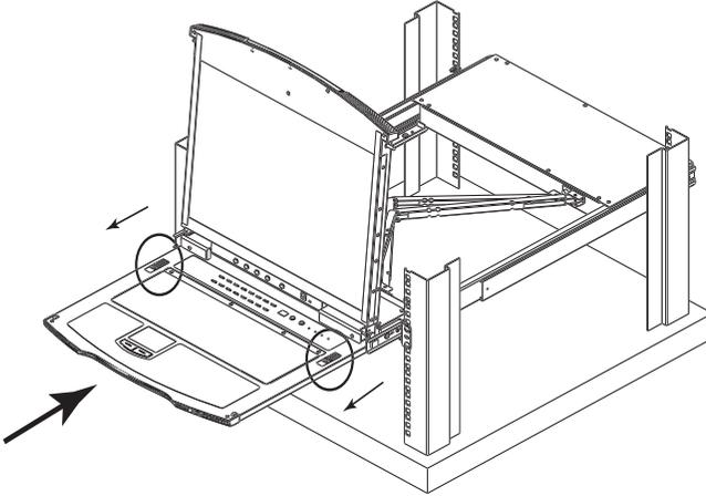
2. Let go of the catches. Using the front handle, push the keyboard module all the way in.
