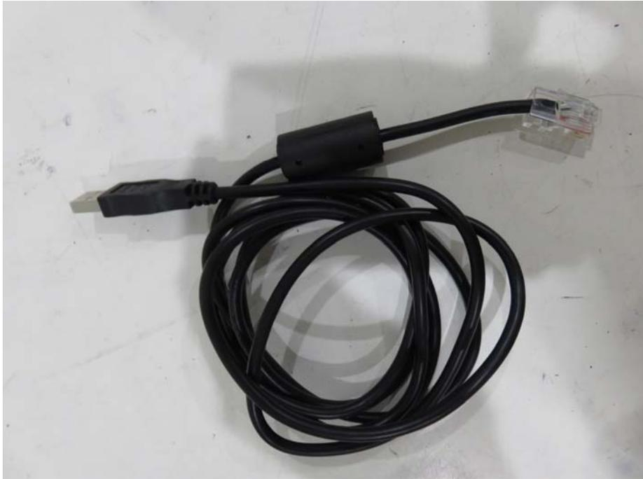
View of the Data Cable (USB to Serial)
