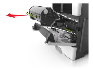
Lift the green handle, and then pull the imaging unit out of the printer.
