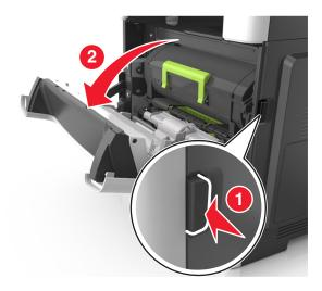
Pull the toner cartridge out using the handle.
