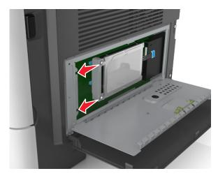
**d** Tighten the two screws.
