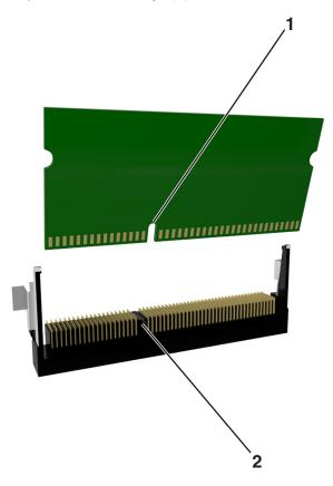
**4** Push the memory card straight into the connector and forward into the controller board wall until it *clicks* into place.
