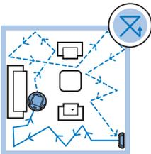
In this mode, the robot cleans the room in a mixed pattern of straight and crisscross movements.
