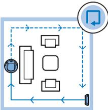
In this mode, the robot follows the walls of the room to give the area alongside the walls an extra clean.
