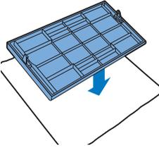
2 Place the dry wipe on a table and place the dry wipe attachment on the wipe with its fixation lugs pointing towards you.
