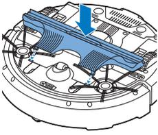
**10** Insert the snap hooks of the TriActive nozzle into the holes in the bottom of the robot. Push the TriActive nozzle back into position. Check if the nozzle can move a few millimeters up and down freely.
