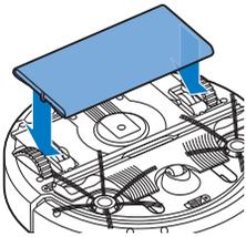
4 Insert the fixation lug of the dry wipe attachment into the opening just behind the wheel on one side of the robot and push until you hear it lock into place with a click. Then repeat these actions on the other side.
