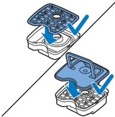
5 Put the filter back into the dust container. Then place the lid on the dust container.
