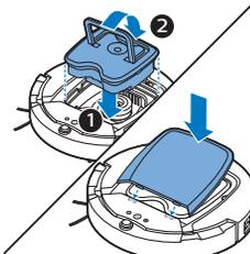
6 Put the dust container back into the dust container compartment (1), fold down the handle (2), and put the top cover back on the robot.
