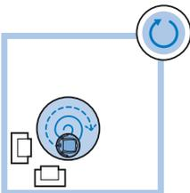
In this mode, the robot moves in a spiral pattern to clean a small dirty area thoroughly. In spiral mode, the fan operates at turbo speed.
