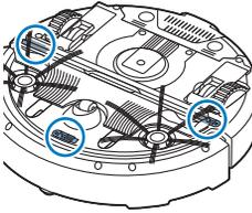
The robot has three drop-off sensors in its bottom. It uses these drop-off sensors to detect and avoid height differences such as staircases.
