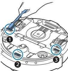
Note: It is important that you clean the drop-off sensors regularly. If the drop-off sensors are dirty, the robot may fail to detect height differences or staircases.
