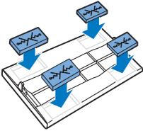
3 Fold both ends of the dry wipe around the dry wipe attachment and fasten the dry wipe onto the attachment by pushing the fixation blocks into the recesses.
