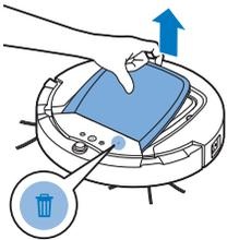
**2** Pull up the handle of the dust container lid and lift the dust container out of the dust container compartment.
