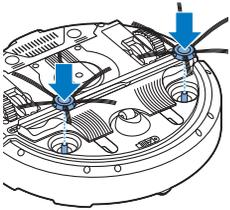
**11** Push the side brushes onto the shafts on the bottom of the robot again.
