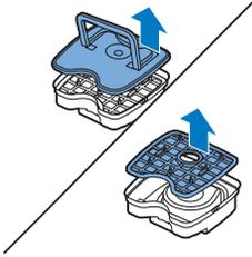
3 Carefully lift the lid off the dust container and take out the filter.
