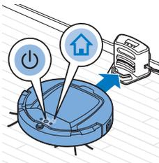
**7** To make the robot return to the docking station before the rechargeable battery runs low, press the docking button on the remote control (FC8932 only). The docking indicator on the display of the robot comes on and the robot returns to the docking station.
