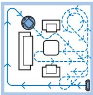
**4** The robot cleans in the auto-cleaning mode until its battery runs low. In the auto-cleaning mode, it follows repeated sequences of Z-pattern, random, wall-following and spiral patterns.
