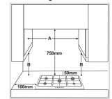
**NOTE:** If the distance "A" between the wall cabinets is between 600 mm and 730 mm, the height "B" must be a minimum of 530 mm. If the distance "A" between the wall cabinets is greater than the width of the hob, the height "B" must be a minimum of 400 mm.
