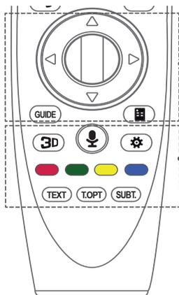
**⌂ Wheel (OK)** Press the center of the Wheel button to select a menu. You can change programmes by using the wheel button.
