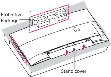
1 When assembling the stand, lay the front screen Protective Package included in the product box on a table or product box and then place the TV screen face down on the Protective Package.
