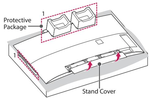
1 When assembling the stand, lay the front screen Protective Package included in the product box on a table or product box and then place the TV screen face down on the Protective Package.
