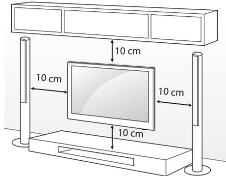
Make sure to use screws and wall mount bracket that meet the standard. Standard dimensions for the wall mount kits are described in the following table.
