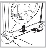
Loosen the drainage pump cover by turning it anticlockwise: it is normal for some water to leak out;
