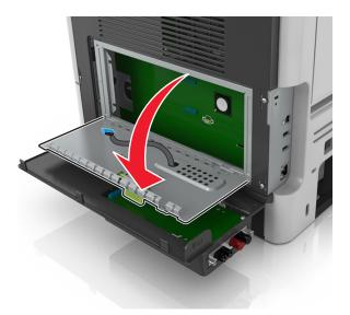
**13** Attach the blue plug of the ISP solution interface cable into the blue receptacle on the controller board.
