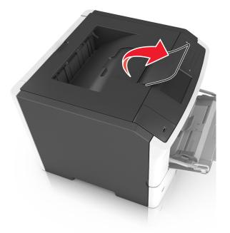
Note: When moving the printer to another location, make sure the paper stop is closed.
