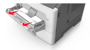
**3** Flex, fan, and align the paper edges before loading.
