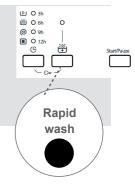
You may make the programme active by pressing the rapid wash auxiliary function button when the led light of the PPI symbol turns on.
