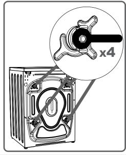
Transportation screws shall be removed by pulling out.
