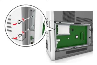
4 Remove the printer hard disk.
