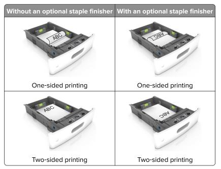
• If you are loading prepunched paper for use with the staple finisher, then make sure the holes on the long edge of the paper are on the right side of the tray.
