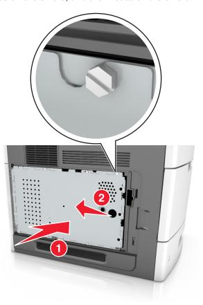
Tighten the screws on the shield.
