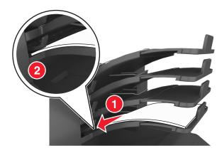
Note: If the paper is not under the bin arm, then a jam occurs due to an overfilled bin.
