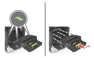
**7** Insert the toner cartridge into the printer by aligning the side rails of the cartridge with the arrows on the side rails inside the printer.
