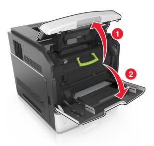
**2** Pull out the toner cartridge from the printer using the handle.
