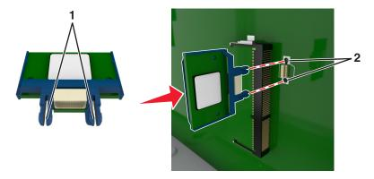
**4** Push the card firmly into place as shown in the illustration.
