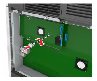
**Note:** Turn the screw clockwise, enough to hold the ISP in place, but do not tighten it yet.
