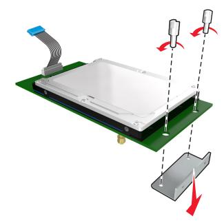
**b** Align the standoffs of the printer hard disk to the holes in the ISP, and then press the printer hard disk down until the standoffs are in place.
