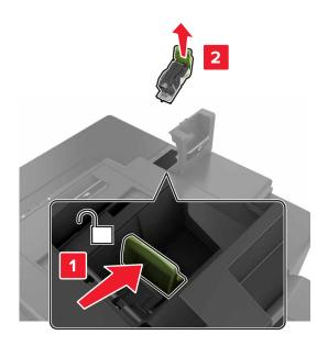
**3** Open the staple guard, and then remove the loose staples.
