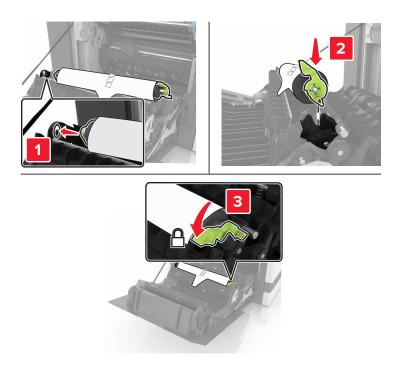
**5** Remove the white packing material.
