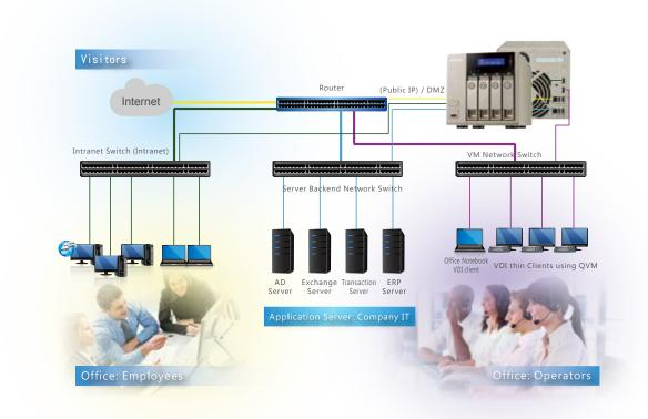
Port Trunking – Link Aggregation for high–speed and high–security file transmission Including the practice mentioned above, 2 LAN ports can be used for Port Trunking – Link Aggregation, enabling IT administrators to set up link aggregation to increase total data transmission capabilities and achieve better efficiency for IT operations. Failover, load balancing, and multi-IP settings are also supported.
