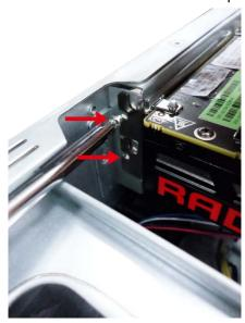
iv. Find the power cable as identified in the below marked area. Connect the power cable to graphic card.
