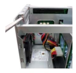
ii. Grasp the edge of the expansion card. Align the notch on the gold edge of the
