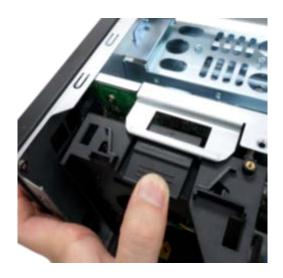
4. Pull the retention clips on each side so that the module can be removed. Remove the installed memory modules.
