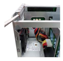
ii. Grasp the edge of the graphics card. Align the notch on the gold edge of the card with the notch in the PCIe slot. Insert the graphics card into the PCIe slot until it cannot go any further.
