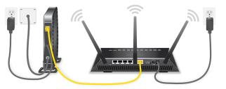
Unplug your modem, remove and replace the backup battery if it uses one, and then plug the modem back in. Use the Ethernet cable to connect the modem to the yellow Internet port on the router.
