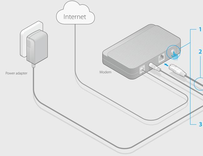
1 Turn off the modem, and remove the backup battery if it has one.
