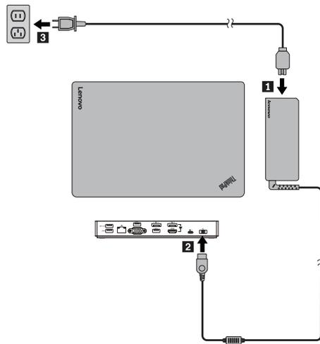
Figure 2. Connecting the dock to the power supply
