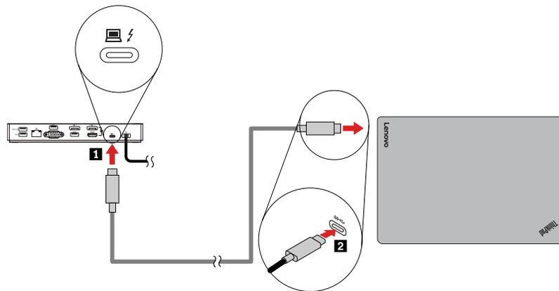
Figure 3. Connecting the dock to the computer
